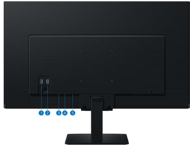
1 USB Type-A Downstream 2 USB Type-A Downstream 3 POWER 4 HDMI IN 1 5 HDMI IN 2 (ARC) / SERVICE
